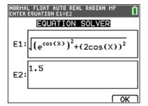
In the Numerical Solver, student enter the left side of the equation as E1 and the right side as E2.
