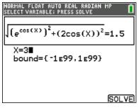
Students then have the ability to set the initial value of xused in searching for the solution as well as set the interval in which the search should be conducted.
